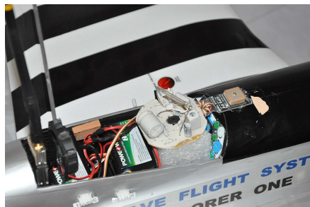
Close up of Beacon Strobe & Video Transmitter
